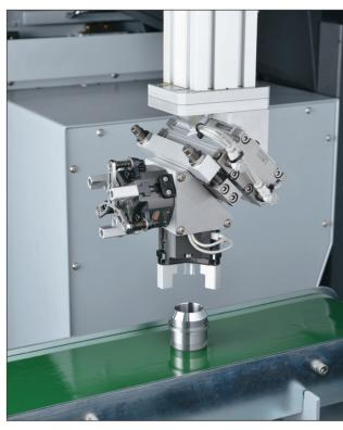
Machine can be equipped with a conveyor
